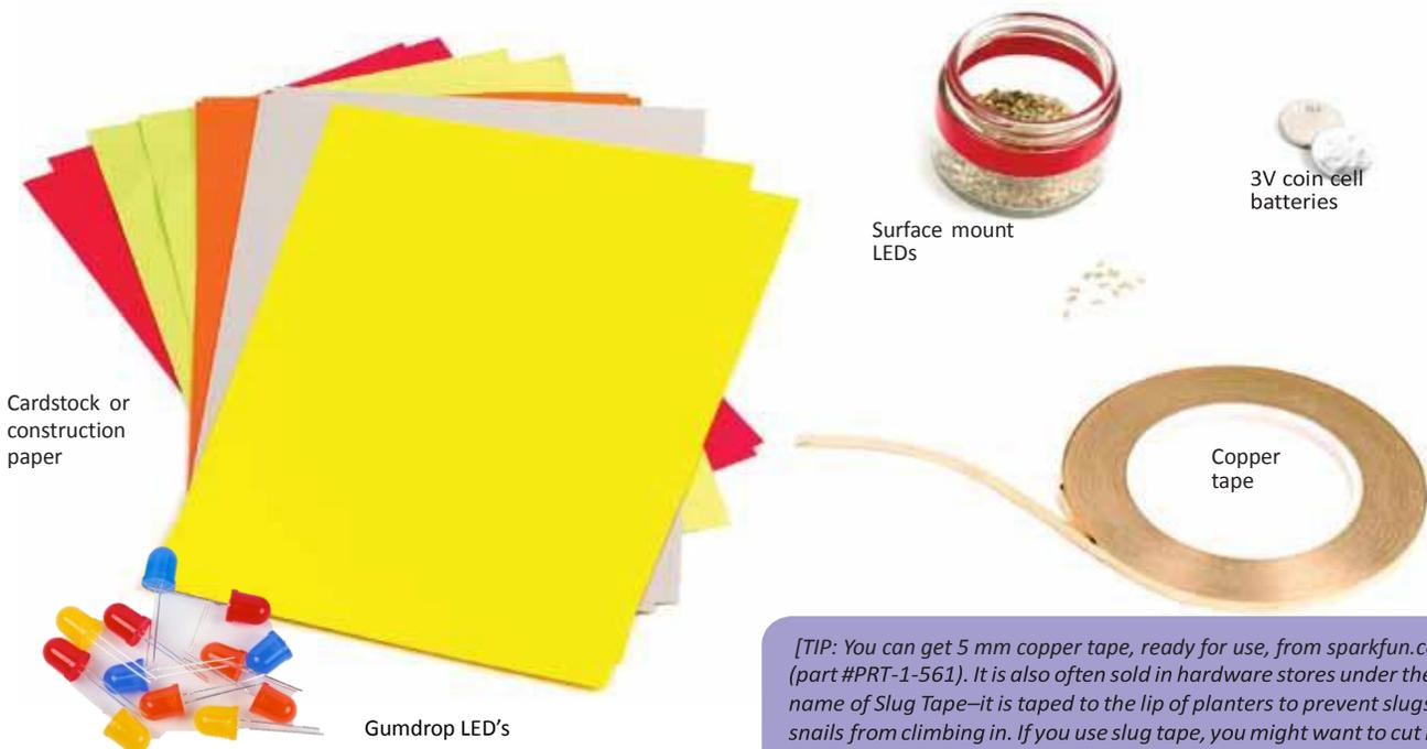
[TIP: You can get 5 mm copper tape, ready for use, from [sparkfun.com](http://sparkfun.com) (part #PRT-1-561). It is also often sold in hardware stores under the name of Slug Tape—it is taped to the lip of planters to prevent slugs and snails from climbing in. If you use slug tape, you might want to cut it into thinner strips before using it on your paper circuit.]
