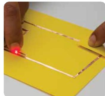
4. Place Scotch tape on the LED (surface mount LED) or on the leads (gumdrop LED) to hold the light in place. You can also solder the LED in place.
