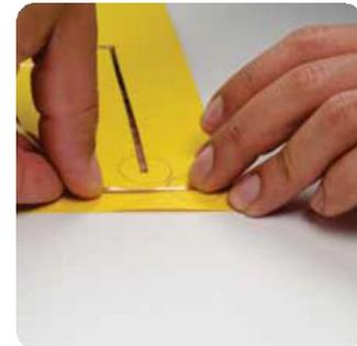
3. Place a gumdrop LED in the gap. Fold the battery in the tab you created earlier and see what happens. You can use a binder clip to hold it in place. Did it light up? If not, what changes can you make to get it to light up?
