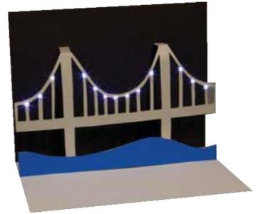
With these materials and the starting instructions, most students will construct a parallel circuit. This allows electrons to travel through multiple paths through the lights. A series circuit has all of the lights in a single row requiring the current to flow through one light in order to reach the next.
